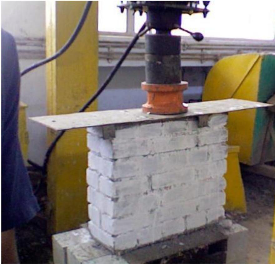
4.1 Prism Test for Fly Ash Bricks
